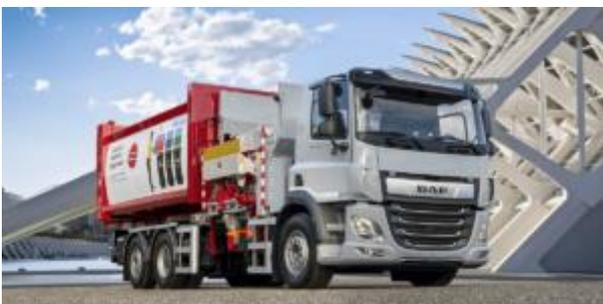
DAF has introduced its first CF Electric truck with a 6x2 rigid chassis.
