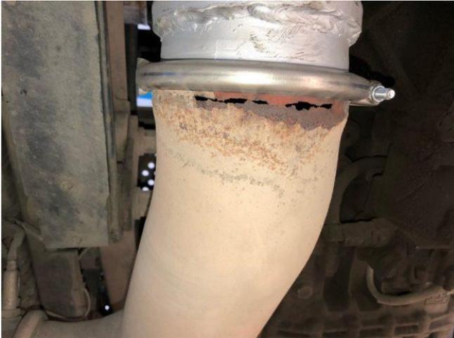
I failed this vehicle – from a main dealer - in the morning for a couple of defects, one being the holes in the exhaust. It came back for retest the same afternoon. The driver was a bit reluctant to put it over the inspection pit.
